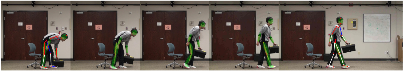
Figure 4: Keyframe based 2D multi-joint tracking: the first and last frames are the annotated keyframe images. The user interactively selects which joints to track and the system automatically tracks their locations at intermediate frames.
